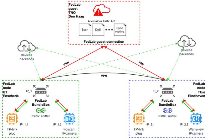
Figure 7. Architecture of the shared experiment using the FedLab. Two Bundle Boxes are deployed in Eindhoven and Enschede, exposing networks hosting two equivalent pairs of IoT devices. Guest access is enabled in Den Haag.
